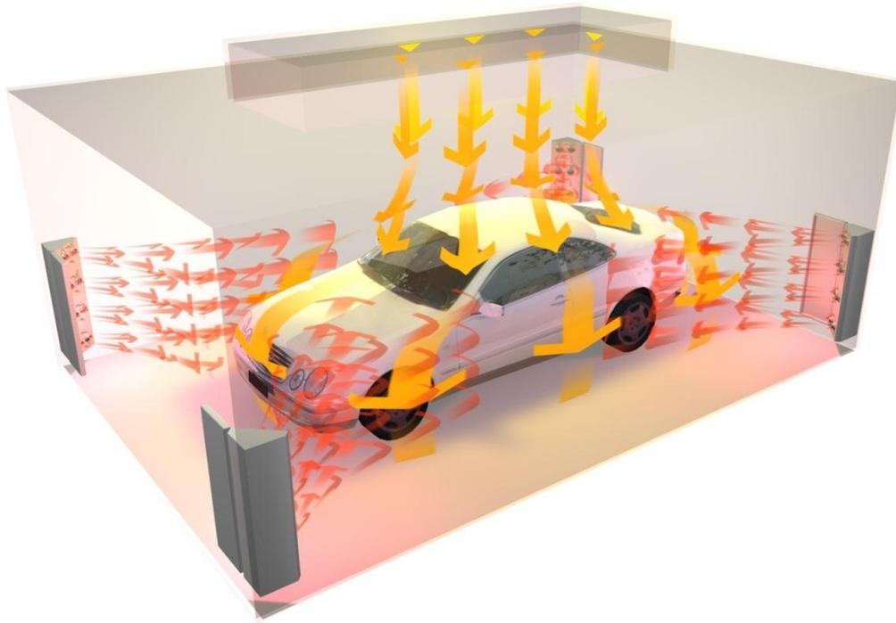
A supplementary air flow is introduced into the spraybooth cabin via high velocity nozzles. This air supply is filtered and heated to the same degree as the spraybooth's conventional airflow. The auxiliary air flow only operates during the flash off and curing cycles.
